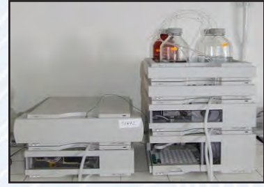
Fig. 120. Cromatograf pe coloana lichida de inalta performanta (HPLC/MWD - Hewlet Packard)
