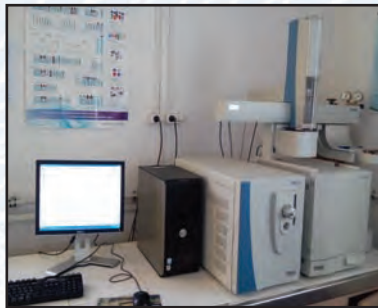
Fig. 139. Gaz cromatograf – Spectrometru de masa – Headspace - Thermo Scientific
